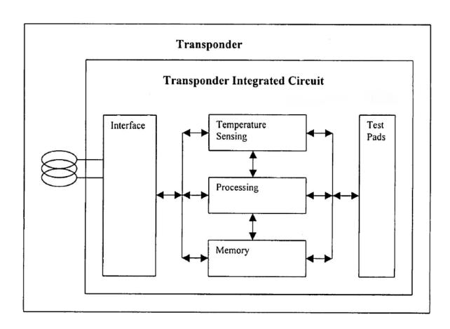
**IMAGE 2** shows the major signals communicated between components of the smart thermometer's temperature sensors.
