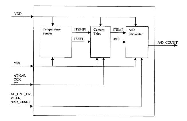
IMAGE 4 is a circuit diagram of the smart thermometer's temperature sensor.
